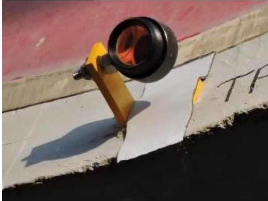
Figure 9.5: Reflective Prism (Tape Fixing)
