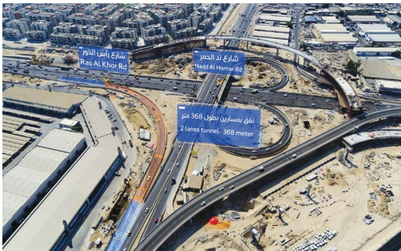
115-metre bridge to serve the traffic inbound from Nadd Al Hamar heading to Ras Al Khor Road in the direction of Dubai-Al Ain Road. A two-lane tunnel extending 368 metres will be constructed to enable right turns from Ras Al Khor Road to Nadd Al Hamar. The project works also include improvements at the existing intersection, and widening the existing turns,” added Al Tayer.
